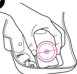
From the underside of the playtray snap the tumbler into place on the two pins as shown.
